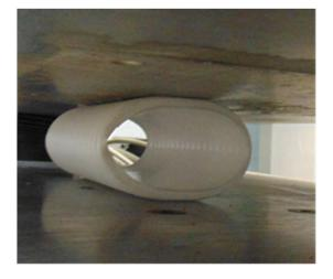
Aircor pipe is tested according to the standard EN ISO 9969 to check deflection with a deformation than 3% the pipe shows no damage to the internal and external wall.
