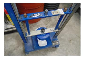
Aircor pipe is tested according to the standard CEI EN 61386-1/-24 to check the ring stiffness with a 5% deformation, higher than 450 N
